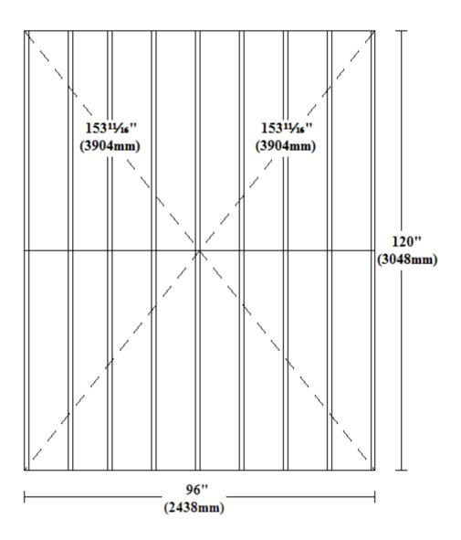
NB:- Floor joists run from gable to gable.
